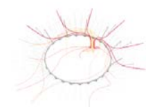
5 branches connect to rear steelwork
